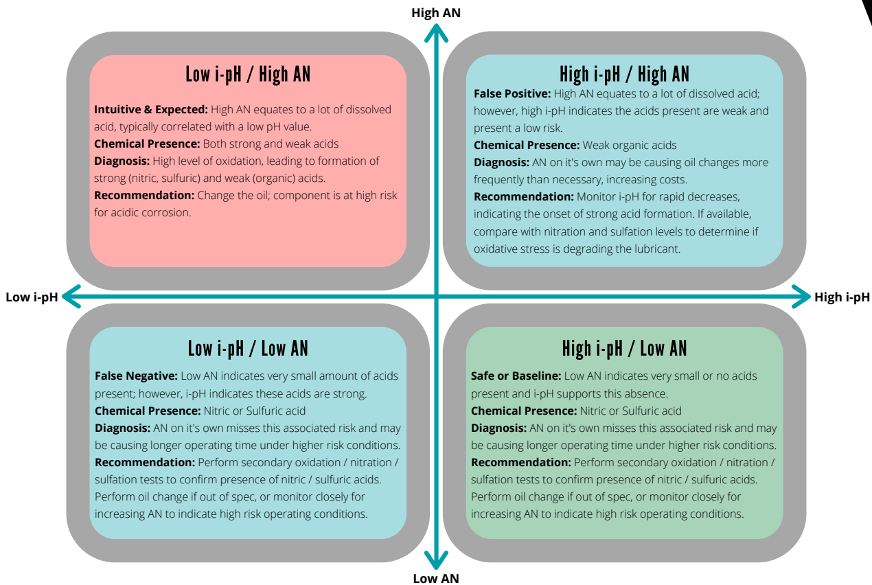
Figure 3: AN vs i-pH regime analysis and interpretations for in-service lubricants.
