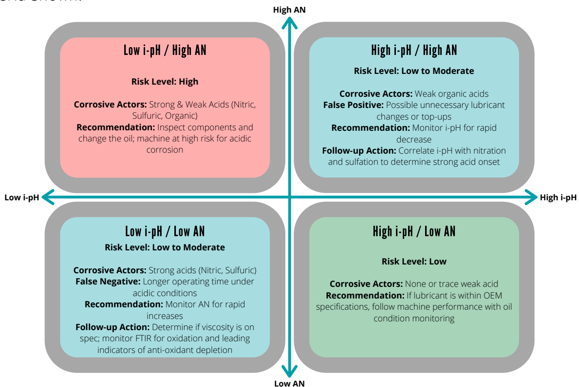
Figure 1: Corrosion risk potential and recommended action based on i-pH/AN quadrants of results
