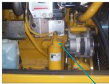
Plug on filter housing
