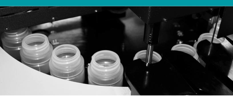
Optical Particle Classification (OPC) is an effective method for determining the particle count and the level of contamination in a lubricating system. OPC testing is ideal for wheel motors, differentials, transmissions, gear boxes, wheel hubs, and final drives.
