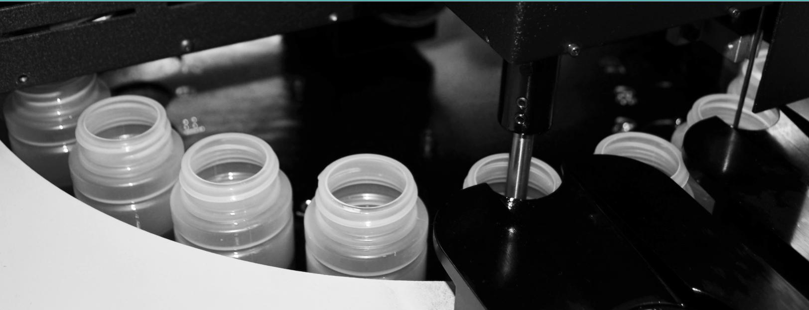
Optical Particle Classification (OPC) is an effective method for determining the particle count and the level of contamination in a lubricating system. OPC testing is ideal for wheel motors, differentials, transmissions, gear boxes, wheel hubs, and final drives.
