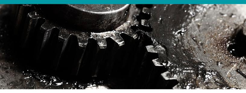
Grease is the preferred choice of lubricant for a variety of situations including: low-speed, back and forth, or minimal bearing rotation; high risk of shock loading / bearing deflection; sealing or leakage control; addressing oil incompatibility issues; or serviceability concerns (i.e. restricted access, remote access). These issues are often the exact failure modes that need to be monitored and controlled.
