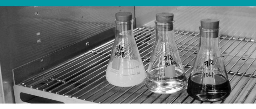
Lubricating oil in hydraulic and gas turbine systems is subject to the effects of varnish. Varnish can be described as thin, oil-insoluble contaminant that is present in the oil and may deposit or plate-out on internal components. Varnish consists of the by-products of oil degradation including oxidation and nitration.
