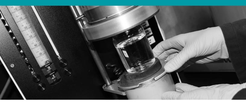
Widely regarded as an important advanced test for oil analysis, it is undeniable that a wide array of historical and potential problems can be quickly be determined by monitoring the number and size-distribution of wear particles and contaminants in a use oil sample. This test cannot be preformed on engine oils or other dark lubricants that do not pass transmitted light.
