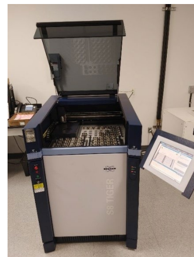
Figure 2. WDXRF Spectrometer used for analysis of Oils and Filter. Source: Fluid Life.
